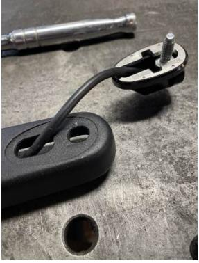
REMOVE THE OEM TURN SIGNAL. INSTALL THE BOLTHEAD IN THE SLOT.
