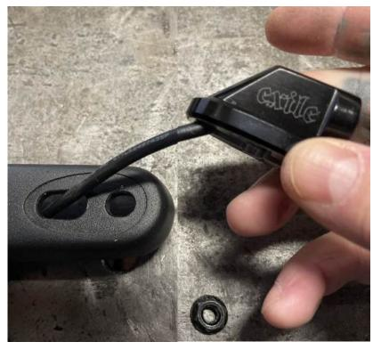
**FOR SOFTAIL-** REMOVE THE STRUT ON ONE SIDE. RUN THE WIRE THROUGH THE FORWARD MOST HOLE.
